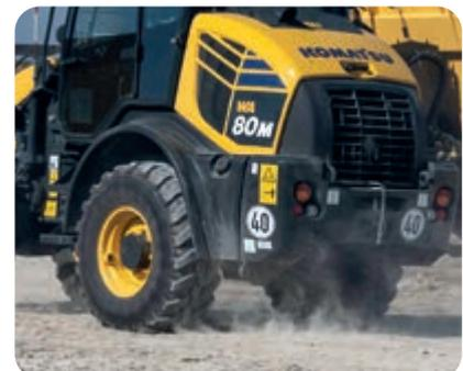
40 km/h limited hydrostatic driveline (option)
