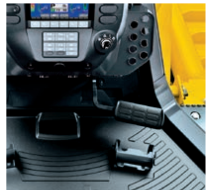
Machine operation is simple with the new one-pedal design that integrates brake function into the decelerator pedal. Machine travel speed can be controlled using one pedal. The pedal function can be changed by a mode selector switch.
