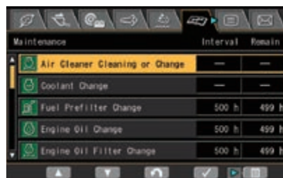
A multifunction monitor displays and controls a wealth of operational and maintenance information
