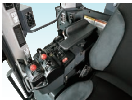
The arm console height can be electrically adjusted
