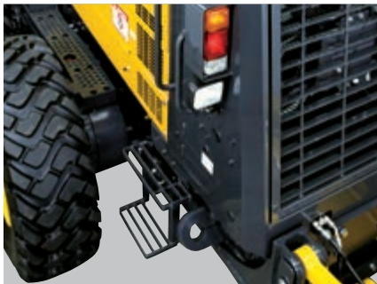
Serrated steps and punched metal foot plate for safe access
