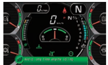
Eco guidance supports energy saving in real time
