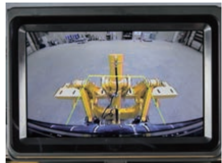
Fully integrated rear-view camera system
